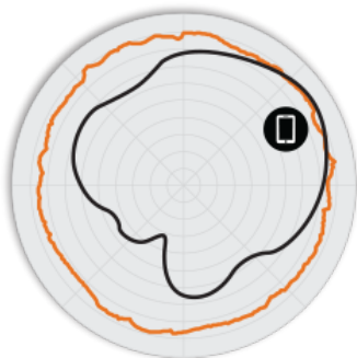
Figure 2. T710o 2.4GHz Azimuth Antenna Patterns
