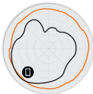
Figure 3. T710o 5GHz Azimuth Antenna Patterns
